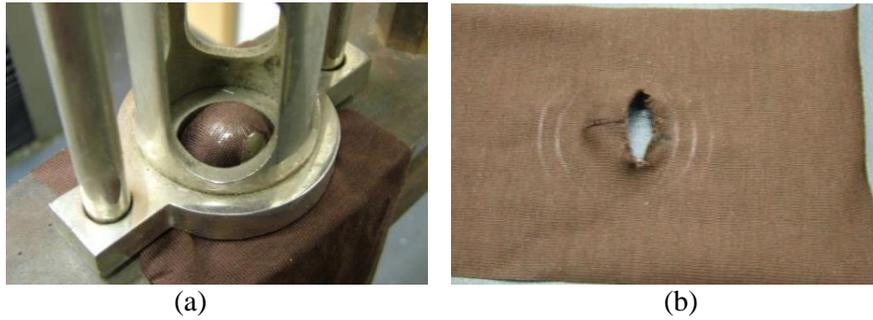
Figure 3: Beginning of the rupture of a knitted lining material (area density: 153 g/m<sup>2</sup>, thickness: 0.42 mm) (a) and the shape and position of the split (b)
